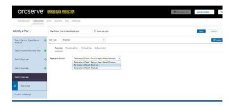
In this configuration, 1:M replication normally must wait until each replicated write completes at each target location. Only after each block of backup data gets written to all replication target locations does the next block of data get replicated. As a result, the replication target location with the highest latency determines the time for the entire replication process to complete.
